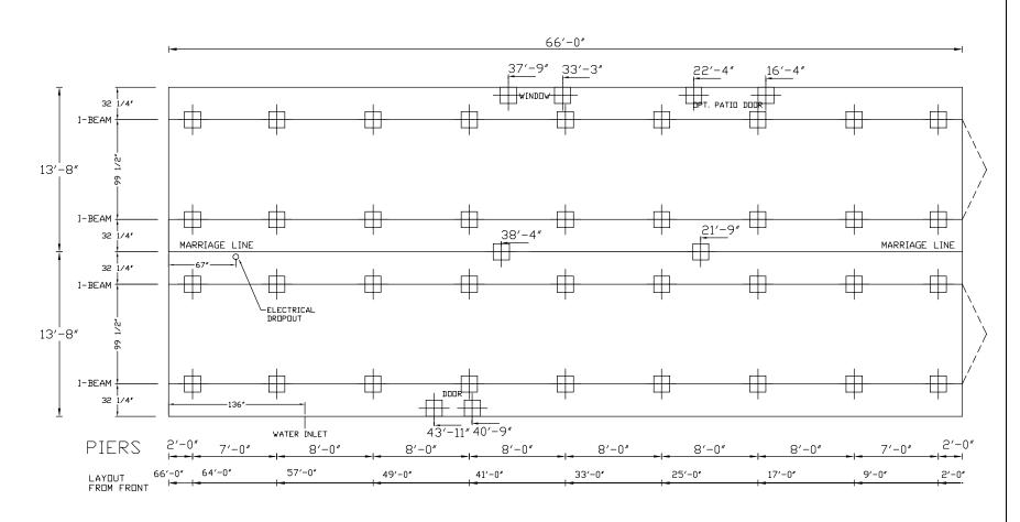
REFER TO LOADING CHART IN INSTALLATION INSTRUCTIONS FOR PIER SPACING PER PAD SIZE BEING USED
